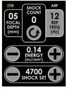
Adaptive Rep Frequency (ARF) Under extreme conditions, such as extended use in a hot environment at the maximum "REP FREQ" and "ENERGY" settings, the CS Pro-VET may automatically reduce the shock wave repetition frequency. This ensures the device always delivers the "ENERGY" value shown on the display. When this occurs, an ARF will be shown at the top of the display, and the sound of shock wave generation will slow down slightly.
