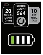
Low Battery B Screen presented while shock is running and battery reaches critically low level. Handheld will power down after shock sequence completes. Charge battery to remedy.
