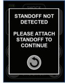
Standoff Missing Message presented when attempting to start shock sequence without standoff connected. Press return to clear message and attach standoff to continue.
